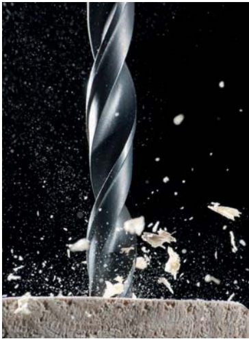
■ Drilling is an example of a cutting process
